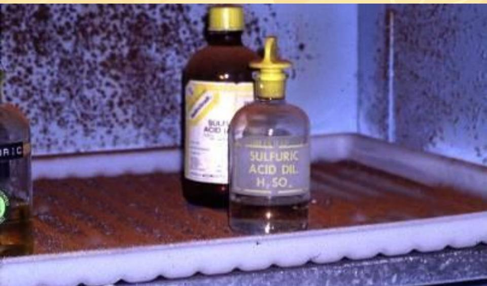
Rusting shelf clips could lead to collapse and acid release
