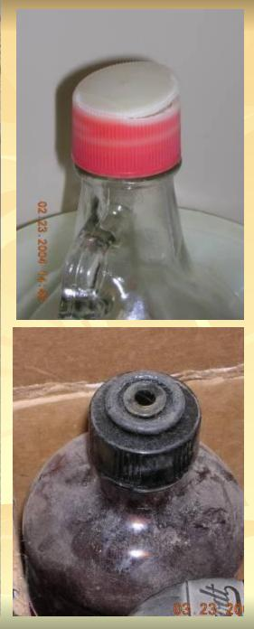
Nitric acid, oxidizer and corrosive. Fumes ate through plastic cap then oxidized cardboard box. Extreme fire risk! Six pounds of cyanide right above it. Earthquake could mean gas chamber for 500 students
