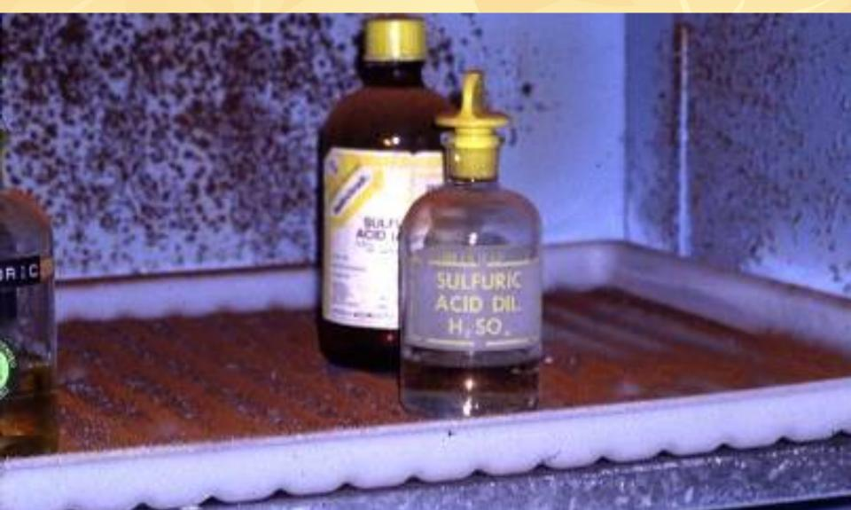
Rusting shelf clips could lead to collapse and acid release
